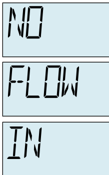
Figure 3-4 NO FLOW IN Alarm
