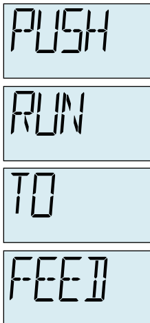
Figure 3-7 PUSH RUN TO FEED Alarm
